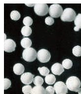
0 50 100μm Powder generated by DL410
