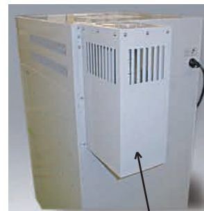
Sample oven with exhaust duct
