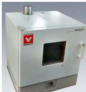
Sample oven with single duct
